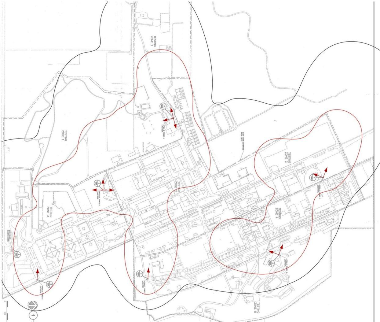
The diagram above shows the system’s acoustic coverage: siren placement and directionality in red, 80 dBC voice contour in orange, and 70 dBC tone contour in blue.
